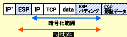
ESP T Tunnel Mode
